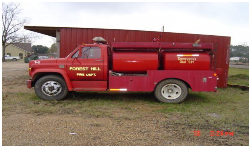
Figure 21: Brush truck configured from FEPP equipment
